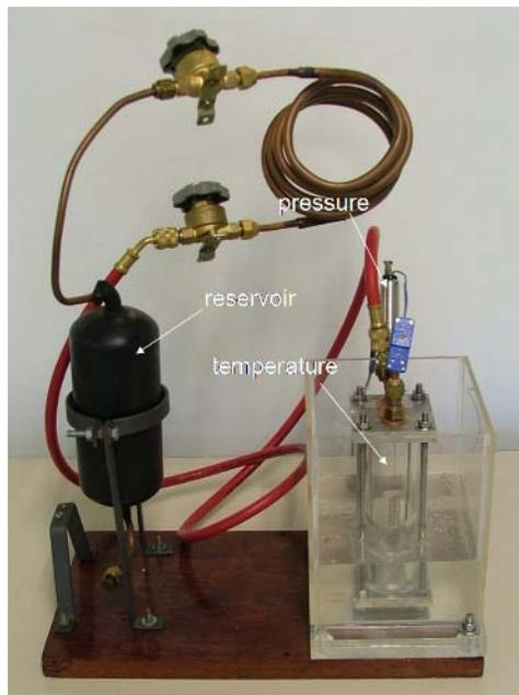
Figure 1. The experimental rig (drawing not to scale).
